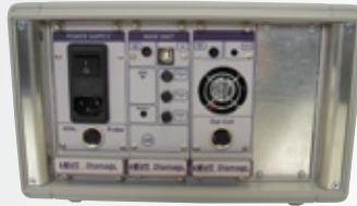
Case: front panel user interface and back panel modules
